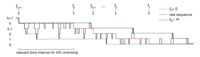
Task. N channels,  $N_0$  locked initially, reconstruct time sequence  $t_{N_0} < t_{N_0-1} < ... < t_k < ... t_1$  of unlocking events. Strategy. The kth channel is considered to become unlocked at the start of a gap to lower conductance levels of duration exceeding a defined cutoff  $\delta_k$ .
